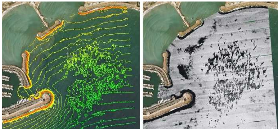
Fig. 4. Left : Isobaths - Right : Corresponding side scan sonar imagery. Black area are full of cymodocea. Dark gray areas contain posidonia.
